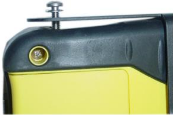
Figure 7. Mounting frame attached to the Titan RT
